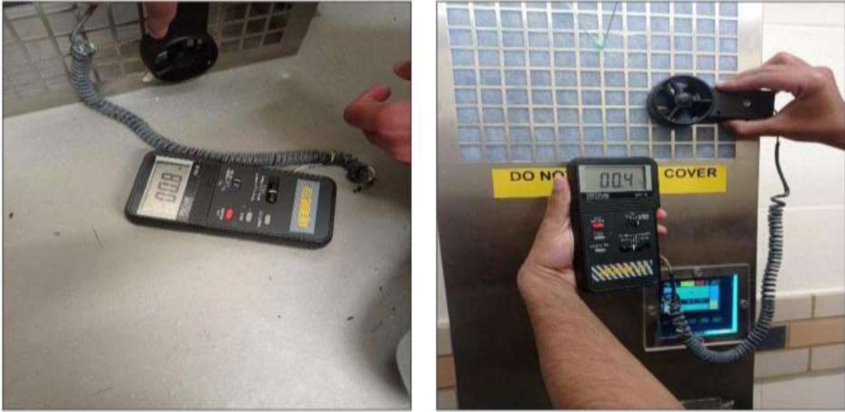
Fig. 2. Air flow measurements using Vane Anemometer in zones 1 and 4.
